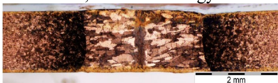
Figure 9 – Cross section welds of Cu-ETP: 1,5 mm, 2 m/min, 60 kV, 130 mA, 10 mm
