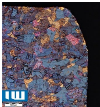
Figure 17 – Micro-section of NVEB-cut of 6 mm thick ETP-copper with 9 m/min at 24.5 kW.( mag.x50)
