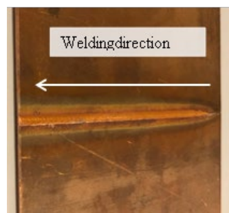
Figure 12 – An inhomogeneous weld of 2 mm Cu-ETP
