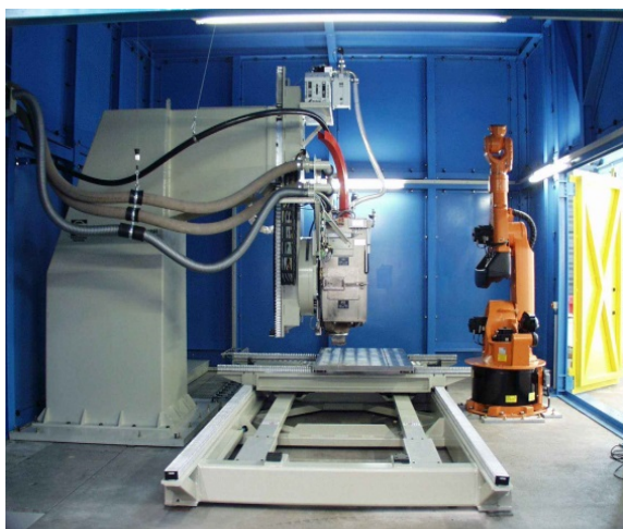
Figure 2 – 175 kV-Non Vacuum Electron Beam Welding machine in the Institute of Materials Science, University of Hanover
