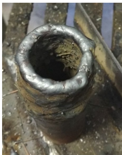
Figure 1 – Additive technology of semi-automatic CO 2 deposition technology to produce cylinder-shaped parts
