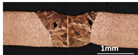
Figure 10 – Cross section welds of Cu-DHP: 0.8 mm, 6 m/min, 60 kV, 120 mA, 6 mm
