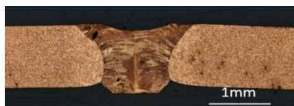
Figure 9 – Cross section welds of Cu-ETP: 1,5 mm, 2 m/min, 60 kV, 130 mA, 10 mm
